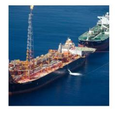
Our Offshore work has certainly kept our development and technical teams on their toes. A Berthing Aid System to monitor dynamic movement of FPSO and Shuttle **Tankers** was delivered for a new-build facility, spread moored in 120m water depth, located on the Mauritania and Senegal maritime border
